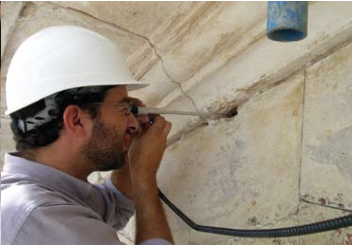
☒ Buroscopia: inspecção no interior das juntas, GCU, 2009 Boroscopy: inspection of interior of joints, GCU, 2009
